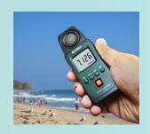
The Extech UV505 pocket-sized UV light meter measures UV-AB light from natural and artificial light sources used in outdoor activities and indoor medical testing, laboratory/research, industrial, education, electronics, and forensics/criminology applications. It offers a backlit display, cosine corrected sensor, two selectable ranges, zero function, display hold, and auto power off. Includes a pouch to protect and store your meter.
