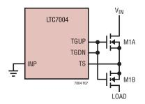
Figure 7. Protecting Load from Voltage Drops on  $V_{\mbox{\scriptsize IN}}$
