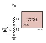
Figure 2. Adjustable OV Lockout
