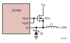
Figure 6. Optional Schottky Diode Usage
