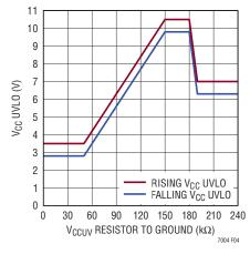
Figure 4. V<sub>CCUV</sub> Resistor Selection
