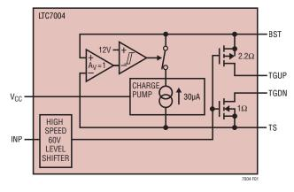
Figure 1. Simplified Output Stage
