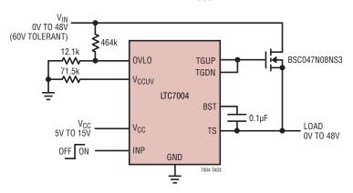
High Side Switch with  $V_{\mbox{CCUV}}$  and  $\mbox{OVLO}$
