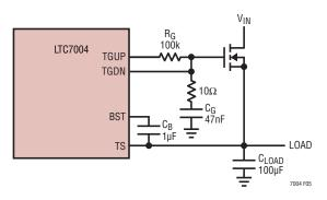
Figure 5. Powering Large Capacitive Loads
