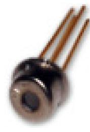
These products are high-performance 850nm VCSELs (Vertical Cavity Surface-Emitting Lasers) designed for high-speed data communications and packaged with a custom designed power monitor diode. The power monitor diode can be used with appropriate feedback control circuitry to set a maximum power level for the VCSEL. These combined features simplify design for high data rate communication and eye safety.
