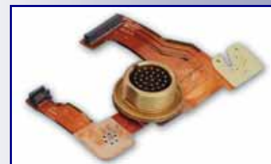
Flex Termination with MIL-C-26482 Special Connector
