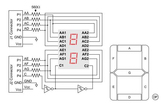
Figure 1. Seven-segment display connection diagram.
