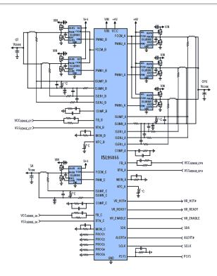
VR C supports 1-phase operation. The address options programmable for these three outputs allow for maximum flexibility in support of the IMVP8™ CPU. All three VRs share a common serial control bus to communicate with the CPU and achieve lower cost and smaller board area compared with a two-chip approach.
