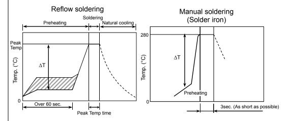
5-3. Recommended soldering peak temp and peak temp duration
