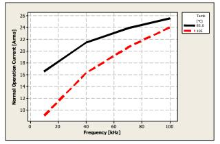
Measurement performed at  $V_{op}$ . The values correspond to a device temperature of +150 °C. No forced cooling was used.
