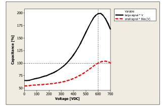
Large signal capacitance: Quasistatic (slow variation of the voltage), +25 °C
