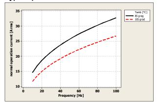
Measurement performed at V<sub>op</sub>. The values correspond to a device temperature of +150 °C. No active cooling was used. Note hat with additional cooling the typical permissible current can be significantly higher.
