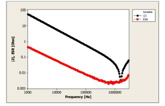
V<sub>DC</sub> = 0 V, V<sub>AC</sub> = 0.5 V<sub>RMS</sub>, T<sub>device</sub> = +25 °C
