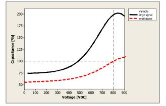
Large signal capacitance: Quasistatic (slow variation of the voltage), +25 °C The nominal capacitance is defined as the large signal capacitance at V<sub>op</sub>. See glossary for further information.
