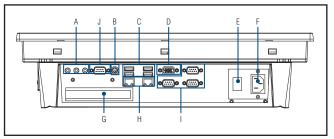
A: Line in/Line out/Mic in B: PS2 Mouse & Keyboard C: USB 2.0 x 4 D: VGA Port E: Power Switch F: AC Inlet G: PCI Slot x 1 H: 10/100/1000 Base-T Ethernet x 2 I: RS-232 x 3 (including RS232/422/485 x 1, COM2) J: RS-232/GPI0 (by swapping pin header)
