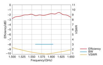
$\bullet$  Tested antenna has been soldered. Evaluation board size is 80x10x1 mm.
