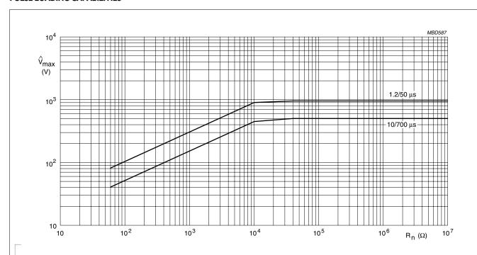
Maximum permissible peak pulse voltage without failing to open circuit' in accordance with DIN IEC 60040 (CO) 533 for type: RC0805
