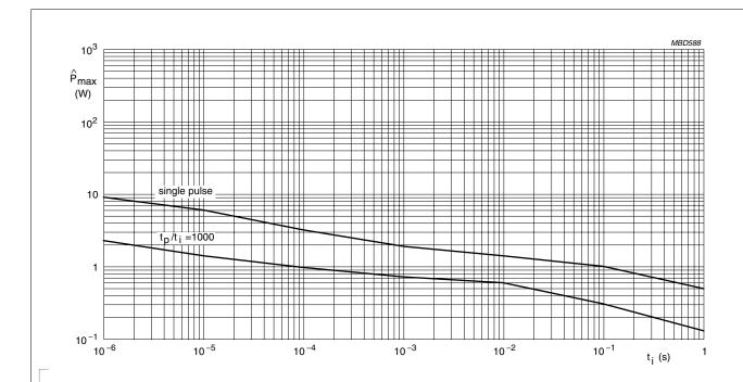
Fig. 7 Pulse on a regular basis for type: RC0805; maximum permissible peak pulse power as a function of pulse duration for single
