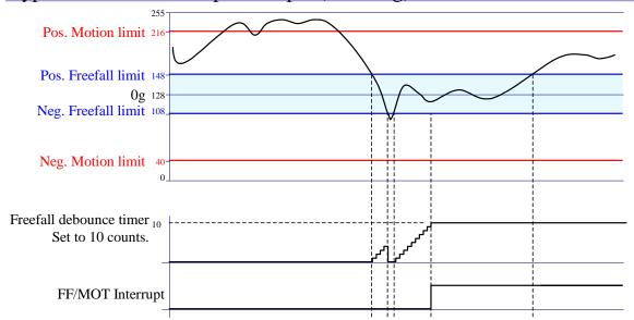
**Figure 15:** Typical Free fall Interrupt Example (FFC ULMODE = 0)
