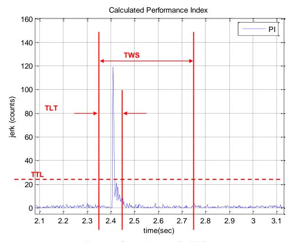
Figure 12: Single Directional TapTM Timing
