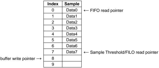
Figure 19: Buffer at Sample Threshold
