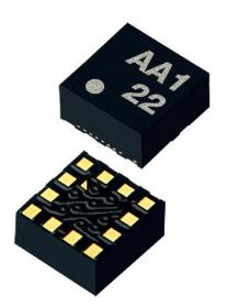
internal operating voltages over the range of input supply voltages. This results in stable operating characteristics over the range of input supply voltages.  $I^2C$  or SPI digital protocol is used to communicate with the chip to configure and check for updates to the orientation, Directional Tap<sup>TM</sup> detection, Free fall detection and activity monitoring algorithms.
