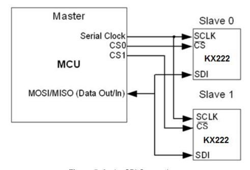
Figure 5: 3-wire SPI Connections
