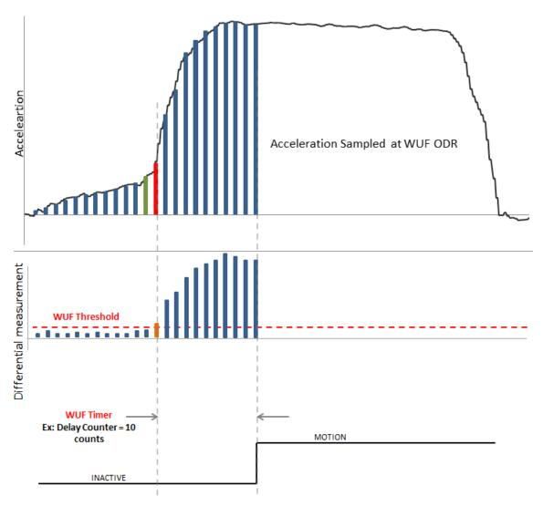
Figure 10: Latched Motion Interrupt Response
