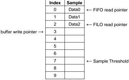
Figure 17: Buffer Filling
