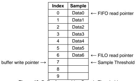
Figure 18: Buffer Approaching Sample Threshold
