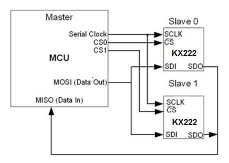
Figure 2: 4-wire SPI Connections
