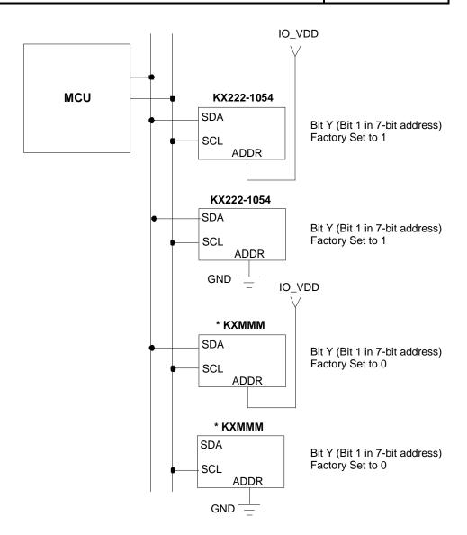
Figure 1: Multiple KX222 Accelerometers on a Shared I<sup>2</sup>C Bus
