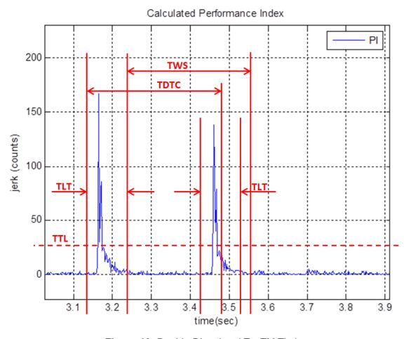
Figure 13: Double Directional TapTM Timing
