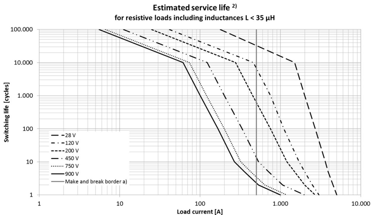
a) Below border make and break operation is permitted, duty cycle 10%, 10 s cycle duration.
