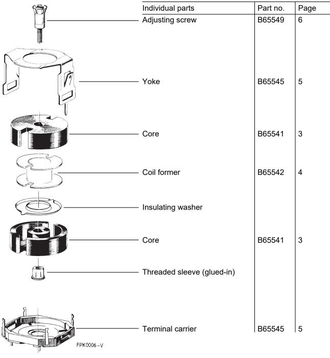
Example of an assembly set for printed circuit boards
