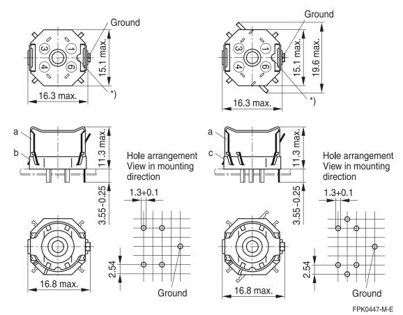
\*) This recess must be on the side of the grounding pin to ensure that the yoke locks in position.
