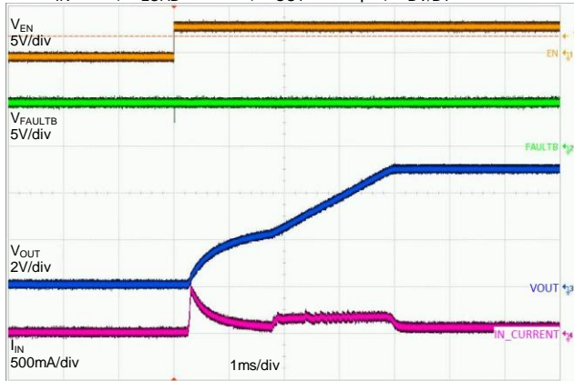
EN Turn ON and In-rush Current at 20V
