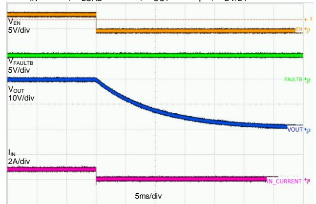
EN Turn OFF with a 5.6Ω Load at 20V
