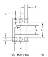
\*Exposed pad P internally connected to pins 2, 3, 4, and 5.
