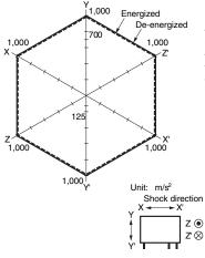
Test Item: G5NB-1A-E, 24VDC Number of Relays: 5 pcs Test Method: Shock was applied 3 times in 6 directions along 3 axes and the level at which shock caused malfunction was measured. Rating: 100 m/s<sup>2</sup>
