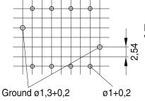
Hole arrangement View in mounting direction
