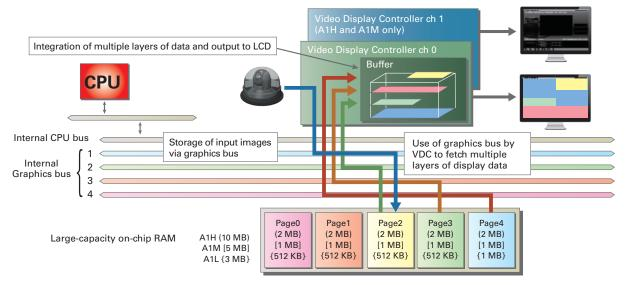
The bus configuration, with independent buses for images and hardware-based superimposition processing, makes it easy to create graphical applications.
