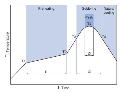
Preheating Soldering Peak Temp. Temp. Time Temp. Time Time Т2 T1 Т4 t1 тз t2 t3 150°C 180°C 60 to 120s 230°C 30s max. 245°C 10s max.
