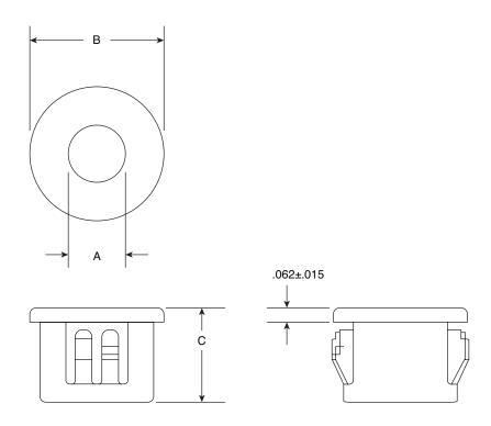
Standard bushings are designed with multiple locks to positively snap in panels ranging from 1/32" to 1/8" thickness. Molded in heat stabilized Nylon UL94V2 black.
