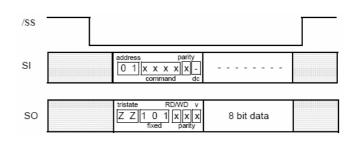
/SS SCK Tristate (Z) SO remains in tristate en address is wrond LSB OUT Bit 13 . х SO ADR0 ADR1 MSB IN: 0 Bit 14: 1 Bit 13 LSB IN .. X SI
