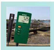
Compact handheld Conductivity Meter with long life carbon rod combination electrode measures Conductivity, TDS and Temperature. Units of measure include  $\mu$ S/cm, mS/cm, ppm, °F, and °C. The meter features three ranges for Conductivity and TDS plus adjustable Temperature compensation factor to maintain accuracy.
