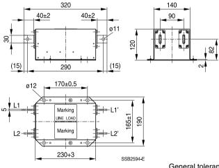
General tolerances according to ISO 2768-cL Dimensions in mm
