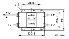
General tolerances according to ISO 2768-cL Dimensions in mm
