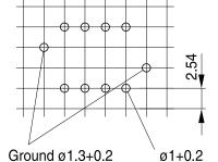
Hole arrangement View in mounting direction
