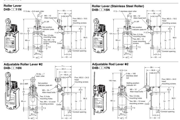
Note: Unless otherwise specified, a tolerance of  $\pm 0.4$  mm applies to all dimensions.
