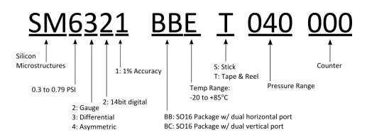
\*Custom calibration pressures and voltages are available to meet specific customer demands. Dual vertical or dual horizontal ports available.
