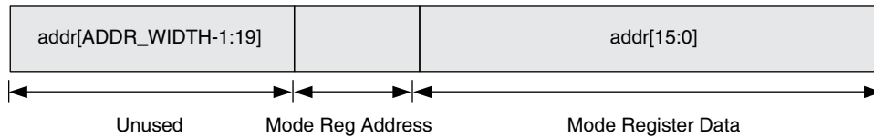
Figure 2-8. User-to-Memory Address Mapping for MR Programming
