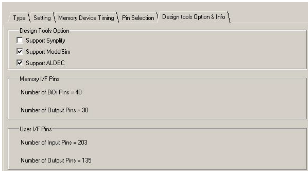
Figure 3-5. DDR3 SDRAM IP Core Design Tools Options and Info Options in the IPexpress Tool
