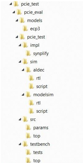
Figure 4.3. LatticeECP3 PCI Express Core Directory Structure
