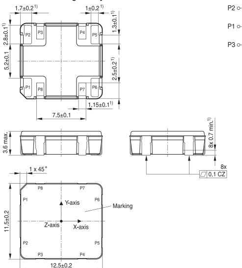
1) Soldering area Dimensions in mm
