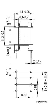
Hole arrangement View in mounting direction
