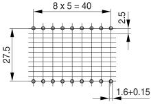
Hole arrangement View in mounting direction
