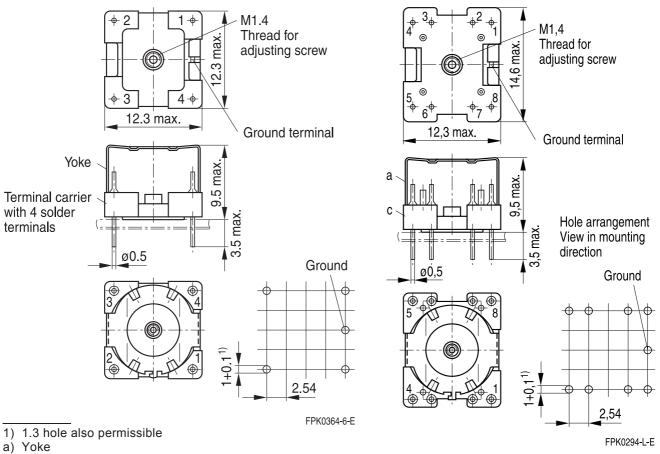
c) Terminal carrier with 8 solder terminals
