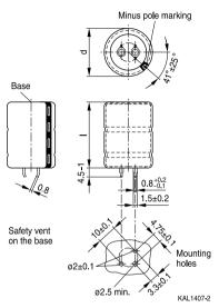
Snap-in capacitors are available with 3 terminals (length (4.5-1) mm). PET insulation is marked with label "PET" on the sleeve.
