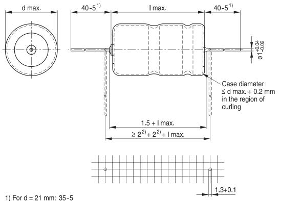
2) Minimum 2 mm bending distance per wire recommended
