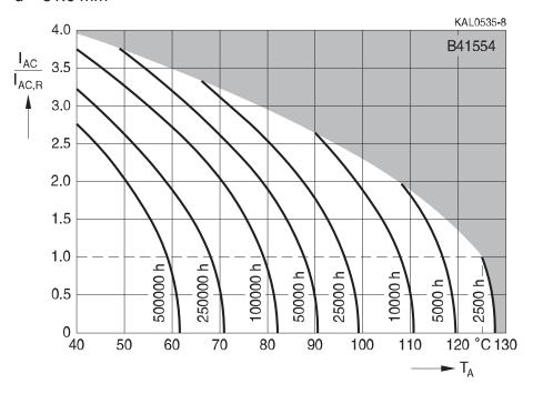
**Useful life** $^{1)}$  depending on ambient temperature  $T_A$  under ripple current operating conditions  $d \geq 64.3 \ mm$
