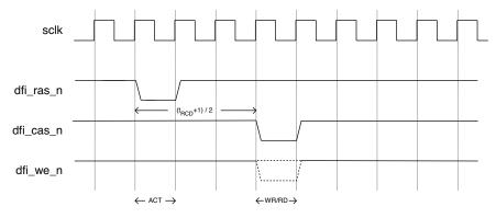
Figure 2-4. Active to Write/Read Command Timing for AL=1 and AL=2
