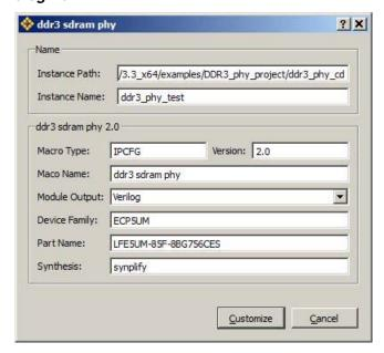
Note that if the Clarity Designer tool is called from within an existing project, Design Location, Device Family and Part Name default to the specified project parameters. Refer to the Clarity Designer tool online help for further information.
