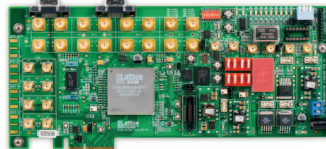
LatticeSC PCI Express x4 Evaluation Board
