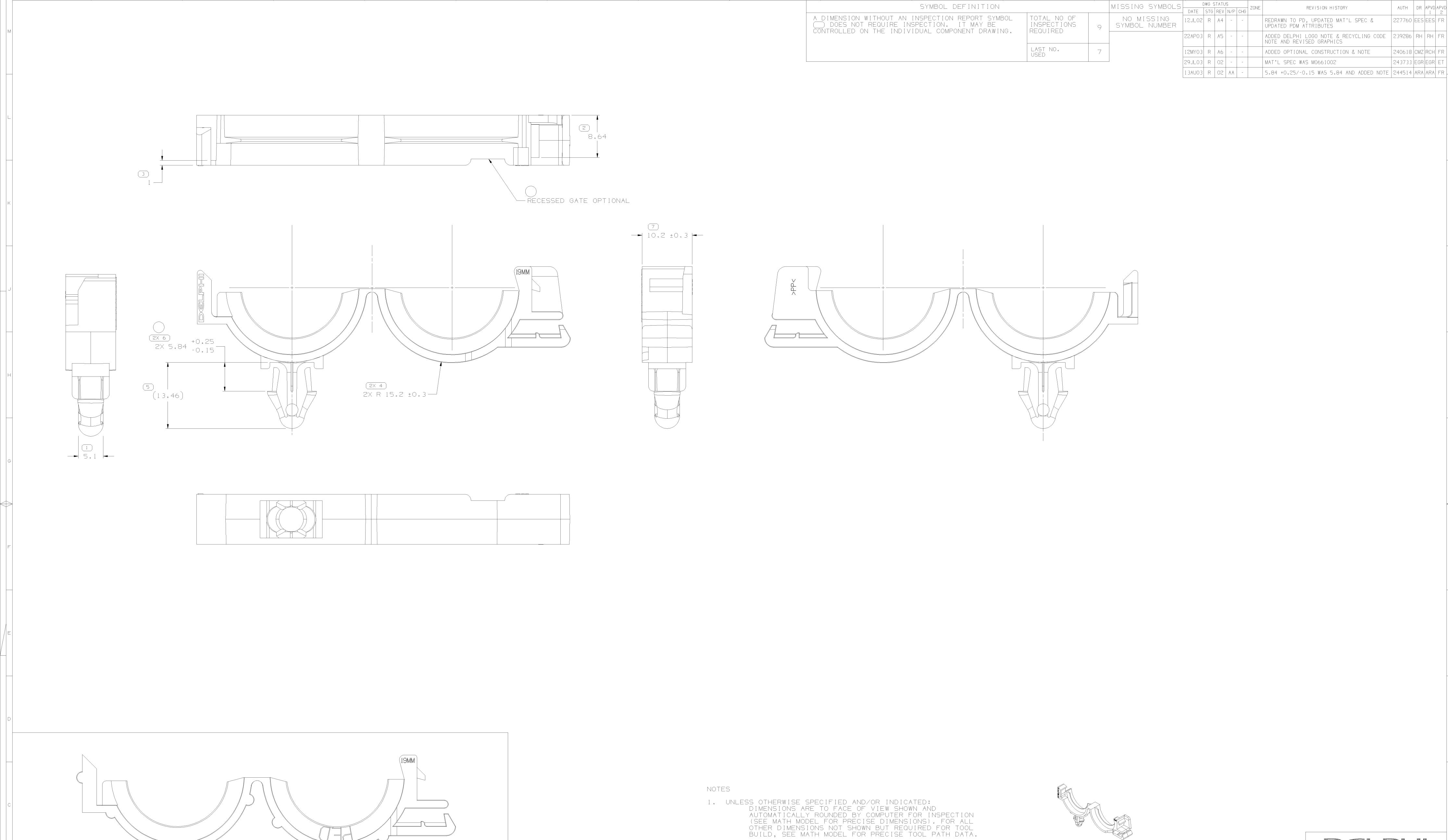
2. MATERIAL RECYCLING CODE >PP< PER SAE JI344. (1)X(0.1) RAISED CHARACTERS AS SHOWN TO BE LOCATED ON ANY EXTERIOR SURFACE.
