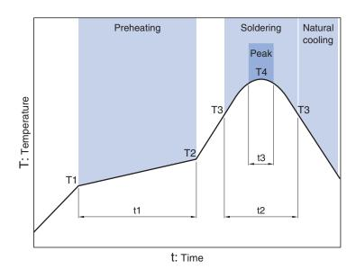
Soldering Preheating Critical zone (T3 to T4) Peak Temp. Time Time Temp. Temp. Time T2 Т3 **T4** t3 150°C 180°C 60 to 120s 230°C 40s max. 260°C max. Within 5s
