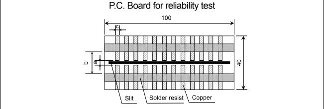
(It is recommended to provide a slit on P.C. board for C3225, C4532 and C5750.) (Unit:mm)
