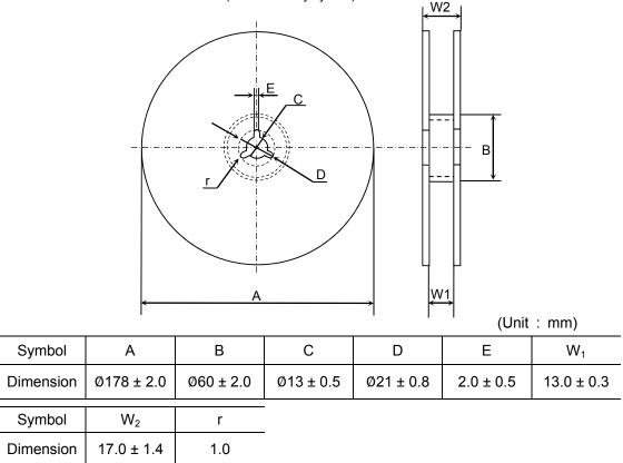
C1005, C1608, C2012, C3216, C3225 ( As for C3225 type, any thickness of the item except 2.5mm ) (Material : Polystyrene)
