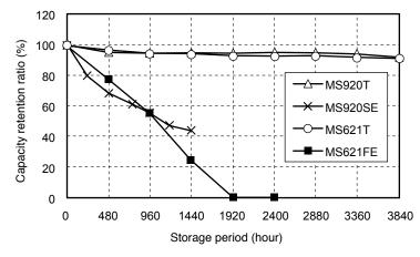
MS-T series's capacity retention ratio after High temperature storage were greatly improved. \* 85°C use of Conventional MS series is not guaranteed.
