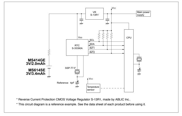
Example of RTC backup time, using MS414GE / MS614SE
