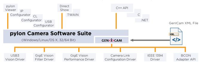
The architecture of the pylon Camera Software Suite is based on GenICam Technology, which offers you easy access to the newest camera models and the latest features. Changes to an existing camera device in your application essentially become a plug-and-play process.
