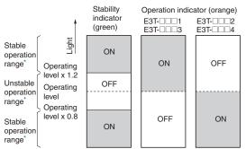
\* If the E3T fs operating level is set to the stable operation range, the E3T will be in most reliable operation without being influenced by temperature change, voltage fluctuation, dust, or setting change. If the operating level cannot be set to the stable operation range, pay attention to environmental changes while operating the E3T.
