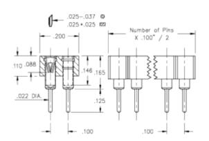
Interconnect Socket Standard Solder Tail Socket Accepts .025"- .037" (0,635 - 0,94 mm)dia leads Double Row Through Hole Plating Code: 47 Shell Plating: 200 µ" Tin (matte finish) over 100 µ" Nickel Inner Contact Plating: Gold Flash
