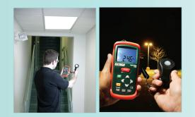
Measures light intensity up to 40,000 Foot-candles or 400,000 Lux with high resolution to 0.01 Fc/Lux. Ideal for indoor lighting tests and for checking security and safety illumination in parking garages, night time ATM areas, stairwells, landings, and hallways.
