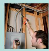
Extech's Video Borescope Inspection Camera with a 4.5mm camera provides a glare-free close-up field of view. It includes a 3.5" color TFT LCD wireless monitor that can be detached from the base and viewed from a remote location up to 32ft (9.75m) from measurement point. Images and videos can be captured with date/ time stamp and played back on the monitor 4-Bright LED Lights
