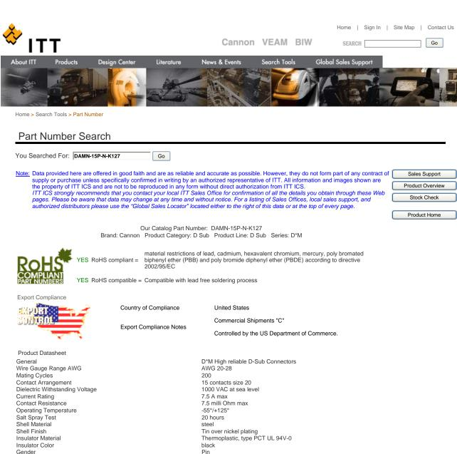
Gender Contact Type Straight PCB Contact Material copper alloy 30 Micro-inch gold
