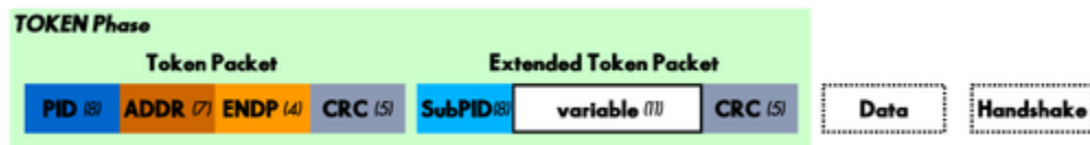
Figure 17 (above) : Extended Token Transaction In an extended token transaction, the token phase of the transaction has two token packets. The first packet uses the EXT PID. The content of the second packet will depend on the particular SubPID specification. The subsequent Data and Handshake phases will depend on the value of the SubPID as well.
