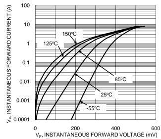
Figure 2. Typical Forward Characteristics
